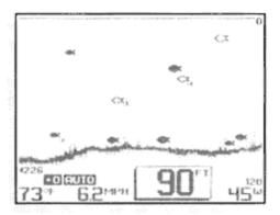
ID is the automatic identification of target returns based on the strength of the returned signal and other factors. Three options are available: ID "On" displays targets as one of three different size fish symbols.
